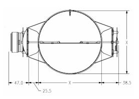
Note: 4"= 100mm NOTE: "X" = 100 TO 225 IN INCREMENTS OF 25mm
