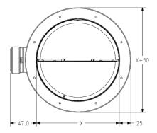
Note: 4" = 100mm NOTE: "X" = 100 TO 225 IN INCREMENTS OF 25mm
