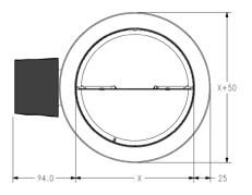
Note: 4"= 100mm NOTE: "X" = 100 TO 225 IN INCREMENTS OF 25mm
