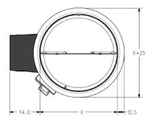
Note: 4"= 100mm NOTE: "X" = 100 TO 225 IN INCREMENTS OF 25mm
