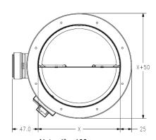
Note: 4" = 100mm NOTE: "X" = 100 TO 225 IN INCREMENTS OF 25mm
