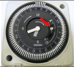
The centre pin in the down '0' position will cause the timer to act as if there we no pins extended.
