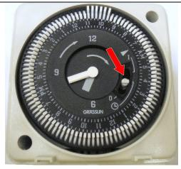
The centre pin placed in the up 'I' position will cause the timer to act as if all the white pins were extended.
