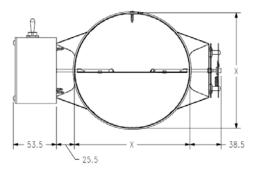
Note 4"= 100mm NOTE: "X" = 100 TO 225 IN INCREMENTS OF 25mm
