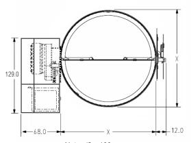
Note: 4" = 100mm NOTE: "X" = 100 TO 225 IN INCREMENTS OF 25mm
