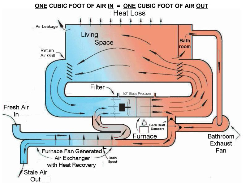
A bathroom exhaust fan has been added and connected to the HAE with two back draft dampers isolating the operation of either the exhaust fan or the furnace fan.
