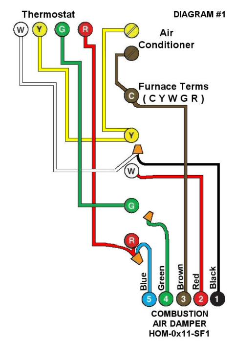
Diagram #1: A Forced Air Furnace or Boiler having a combustion air supply duct.
