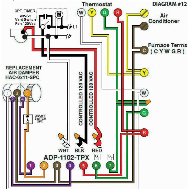
**Diagram #12:** Forced Air Furnace having a **replacement air** supply duct together with a designated **ventilation switch** and/or **bathroom timer** to turn on an **exhaust fan INTERLOCKED** to a replacement **air control damper**.
