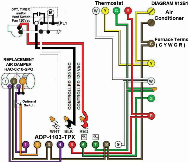
**Diagram #12B1:** Forced Air Furnace having a **replacement air** supply duct together with a designated **ventilation switch** and/or **bathroom timer** to turn on an **exhaust fan INTERLOCKED** to a replacement **Power Open air control damper**.
