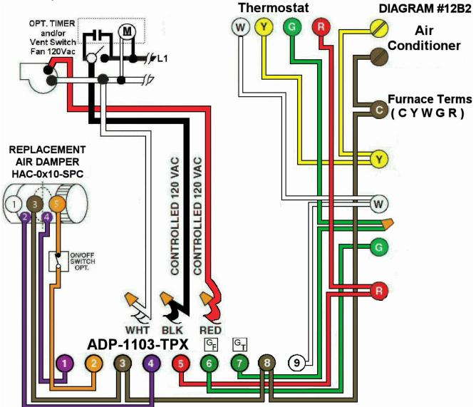
**Diagram #12B2:** Forced Air Furnace having a **replacement air** supply duct together with a designated **ventilation switch** and/or **bathroom timer** to turn on an **exhaust fan INTERLOCKED** to a replacement **Power Closed air control damper**.
