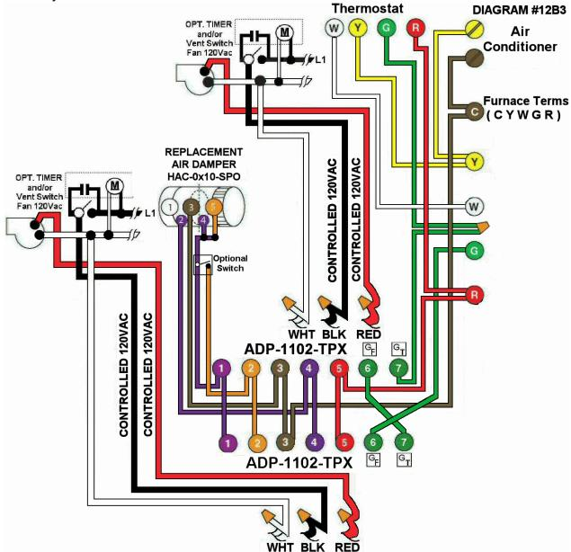
**Diagram #12B3:** Forced Air Furnace having a **replacement air** supply duct together with **two** designated **ventilation switches** and/or **bathroom timers** to turn on an **exhaust fan INTERLOCKED** to a replacement **Power Open air control damper.**
