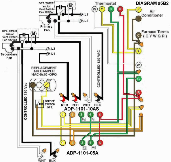
**Diagram #5B2:** Forced Air Furnace having one **replacement air** supply duct together with <u>two</u> **exhaust fans,** one primary that overrides the secondary, both controlled by <u>two interlocking</u> relay adaptors, one being **ADP-1101-10AS and the other ADP-1101-05A**.
