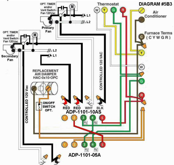
**Diagram #5B3:** Forced Air Furnace having one **replacement air** supply duct together with **two exhaust fans**, one Primary that overrides the secondary, both controlled by **two interlocking** relay adaptors, one being **ADP-1101-10AS** and the other **ADP-1101-05A**.
