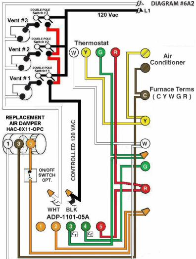
**Diagram #6A2:** Forced Air Furnace having a **replacement air** supply duct together with **two** (or more) **exhaust fans** controlled by **two** (or more) **separate Double Pole Ventilation switches\***.
