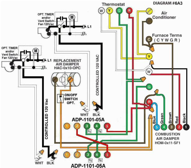
**Diagram #6A3:** Forced Air Furnace having a **combustion air** and a **replacement air** supply duct together with **two exhaust fans** controlled by **two** relay adaptors (**ADP-1101-05A**).
