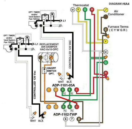
**Diagram #6A4:** Forced Air Furnace having one **replacement air** supply duct together with **two exhaust fans** controlled by **two** relay adaptors, one being **ADP-1101-05A** and the other **ADP-1102-TWP**.
