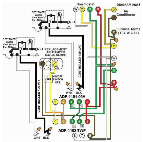
**Diagram #6A5:** Forced Air Furnace having one **replacement air** supply duct together with **two exhaust fans** controlled by **two** relay adaptors, one being **ADP-1101-05A** and the other **ADP-1102-TWP**.
