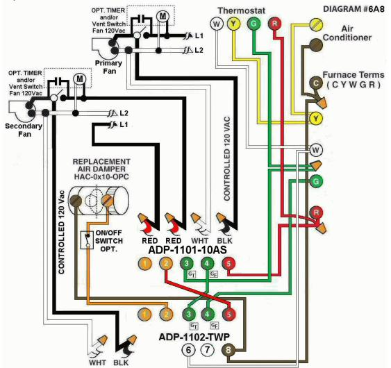
**Diagram #6A8:** Forced Air Furnace having one **replacement air** supply duct together with <u>two</u> **exhaust fans,** one Primary that overrides the secondary, both controlled by <u>two interlocking</u> relay adaptors, one being **ADP-1101-10AS and the other ADP-1102-TWP.**
