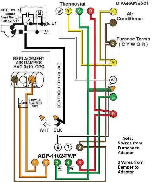
**Diagram #6C1:** Forced Air Furnace having a **replacement air** supply duct together with and **exhaust fan** controlled by a designated **ventilation switch and/or bathroom timer**.
