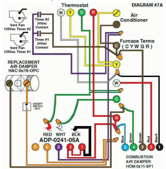
**Diagram #7A:** A Forced Air Furnace, a **combustion air** supply duct, a **replacement air** supply duct, **two exhaust fans.** two **individual timers** and an adaptor **ADP-0241-05A.**
