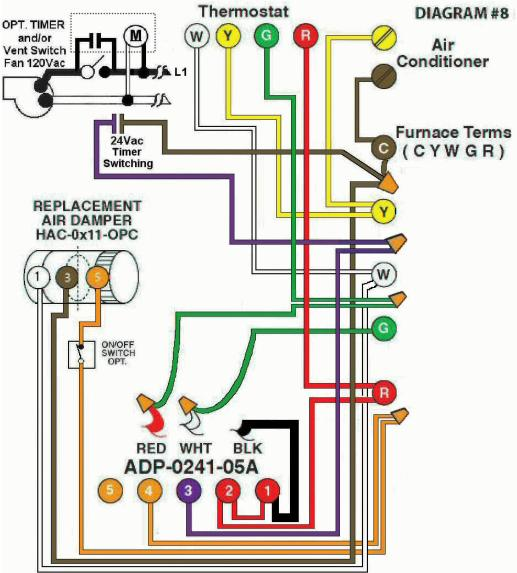
**Diagram #8:** Forced Air Furnace having a **replacement air** supply duct together with an **exhaust fan** controlled by a **designated ventilation switch and/or bathroom timer** that sends a 24Vac signal to the furnace area.
