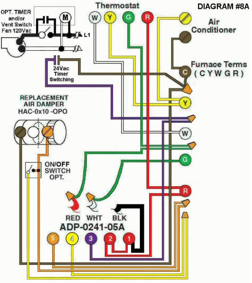
**Diagram #8A:** Forced Air Furnace having a **replacement air** supply duct together with an **exhaust fan** controlled by a **designated ventilation switch and/or bathroom timer that sends a 24Vac signal** to the furnace area.
