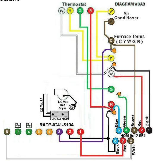
**Diagram #8A3:** A Forced Air Furnace having a **combustion air** supply duct that also serves as a combustion air supply for a 120Vac gas dryer as a secondary appliance.
