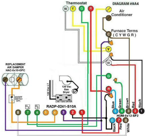
**Diagram #8A4:** A Forced Air Furnace having a **combustion air** supply duct and also a **replacement air** supply duct that provides additional air for a 120Vac **gas dryer** and for the normal operation of the home.
