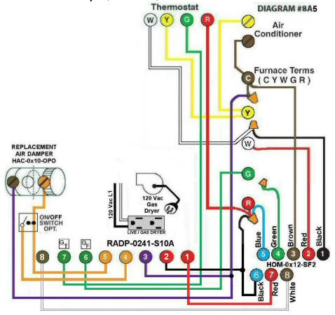
**Diagram #8A5:** A Forced Air Furnace having a **combustion air** supply duct and also a **replacement air** supply duct that provides additional air for a 120Vac **gas dryer** and for the normal operation of the home.
