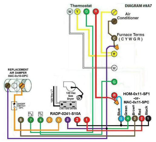
**Diagram #8A7:** Forced Air Furnace having a **replacement air** supply duct directed into the return plenum which provides fresh air for the living area in the home. Also included is a **separate fresh air duct** for a 120Vac **Gas Dryer**.
