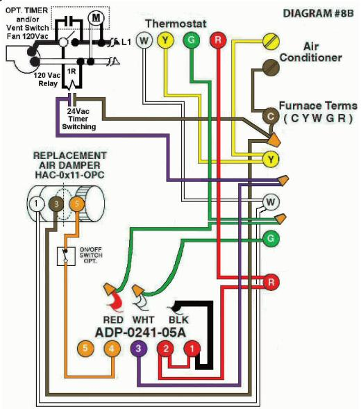
**Diagram #8B:** Forced Air Furnace having a **replacement air** supply duct together with an **exhaust fan** controlled by a **designated ventilation switch** and/or **bathroom timer**.
