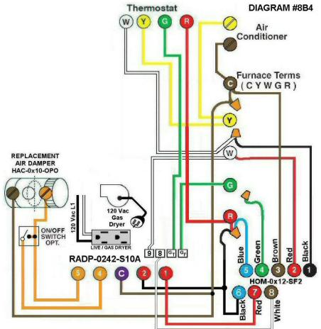
**Diagram #8B4:** A Forced Air Furnace having a **combustion air** supply duct and also a **replacement air** supply duct that provides additional air for a 120Vac **gas dryer** and for the normal operation of the home.
