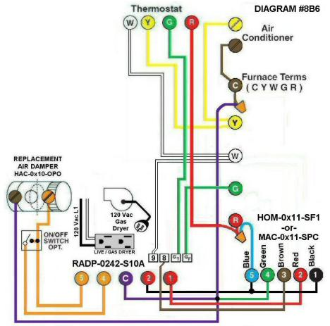
**Diagram #8B6:** Forced Air Furnace having a **replacement air** supply duct into the return plenum which provides fresh air for the living area in the home. Also included is a **separate fresh air duct** for a 120Vac **Gas Dryer**.
