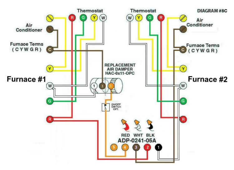
**Diagram #8C: Two** Forced Air Furnaces sharing a common **replacement air** supply duct controlled by one **Power Close** fresh air damper with a **Relay**. The damper opens when either furnace fires. If using a **Power Open** damper, go to wiring Diagram # **8C1** for details.
