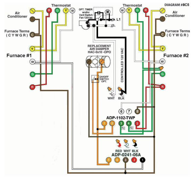
**Diagram #8C5: Two** Forced Air Furnaces sharing a common **replacement air** supply duct equipped with one **P**ower **O**pen fresh air damper. A **designated ventilation switch** and/or **bathroom timer** interconnected to an **ADP-1102-TWP** acting as a control centre for one furnace and an **ADP-0241-05A** interconnected and acting as a control centre for the other furnace.
