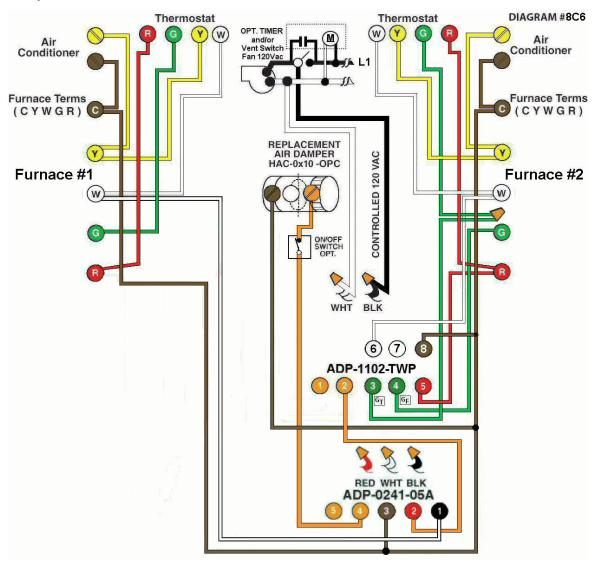
**Diagram #8C6: Two** Forced Air Furnaces sharing a common **replacement air** supply duct equipped with one **Power Close** fresh air damper. A **designated ventilation switch** and/or **bathroom timer** interconnected to an **ADP-1102-TWP** acting as a control centre for one furnace and an **ADP-0241-05A** interconnected and acting as a control centre for the other furnace.
