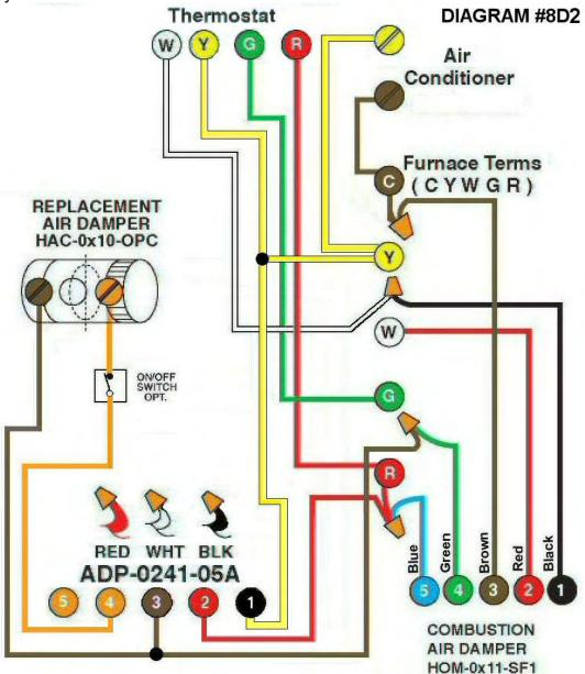
**Diagram #8D2:** Forced Air Furnace with a fresh air supply duct for **combustion air** and a **replacement air** supply duct.
