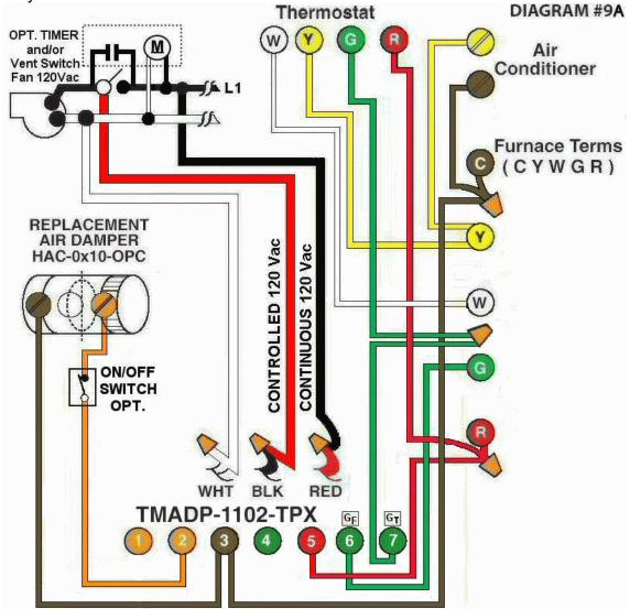
**Diagram #9A:** Forced Air Furnace having a **replacement air** supply duct together with an **exhaust fan** controlled by a designated **ventilation switch** and/or an **optional bathroom timer** and an **interval timer**.
