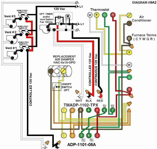
**Diagram #9A2:** Forced Air Furnace having a **replacement air** supply duct together with **two** (or more) **exhaust fans** controlled by **two** (or more) **separate Double Pole Ventilation Switches**.
