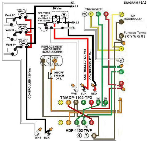
**Diagram #9A5:** Forced Air Furnace having a **replacement air** supply duct together with **two** (or more) **exhaust fans** controlled by **two** (or more) **separate Double Pole Ventilation Switches**, a **Timer Adaptor** and an **Adaptor** control by the **thermostat**.
