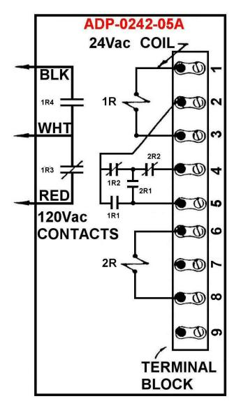
Note: This marking is also on the cover of the Adaptor unit as well as on a label to be placed next to the wiring diagram of the appliance. Schematic Wire Diagram of ADP-0242-05A Activated by an Exhaust Fan Auxiliary Relay Switch 24Vac or manual switch to simultaneously turn on an exhaust fan, a furnace circulating fan and open a Fresh Air damper. The second Relay actuates the fresh air damper during the heating cycle of the furnace.
