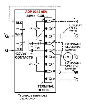
Suggestion: Use fresh air damper HAC-0X10-OPO/PC. X = Diameter of damper, PO= Power Open, PC= Power Close.
