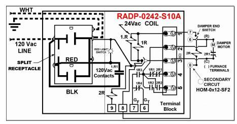
This label is to be placed on the Appliance using Damper HOM-0x12-SF1
