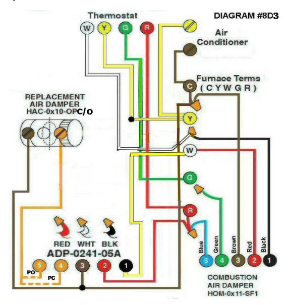
**Diagram #8D3:** Forced Air Furnace with a **combustion air** damper and a separate air supply duct for a **replacement air** Damper, both to open during firing of the furnace.
