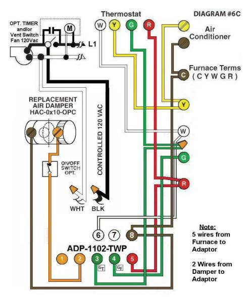
**Diagram #6C:** Forced Air Furnace having a **replacement air** damper together with and **exhaust fan** controlled by a designated **ventilation switch and/or bathroom timer**.
